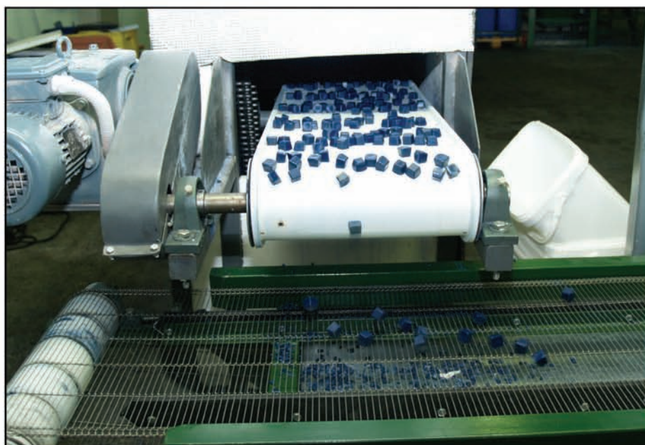
Rodenticide wax blocks roll off the line
